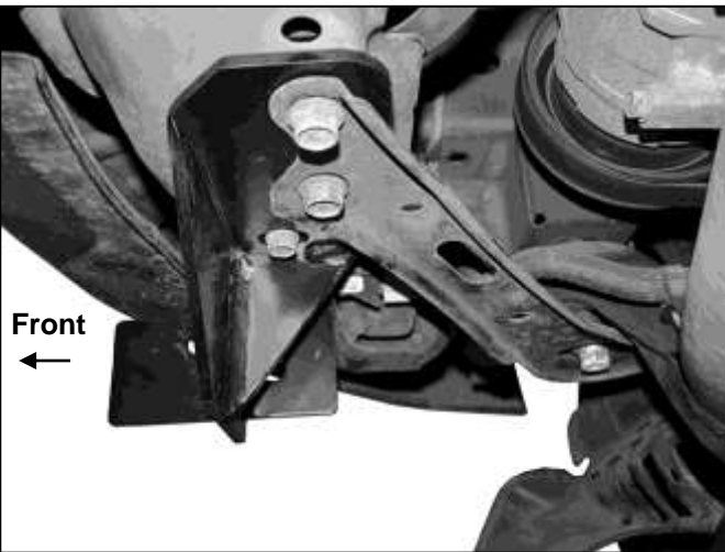
(Fig 3) Passenger/right Mounting Bracket installed
