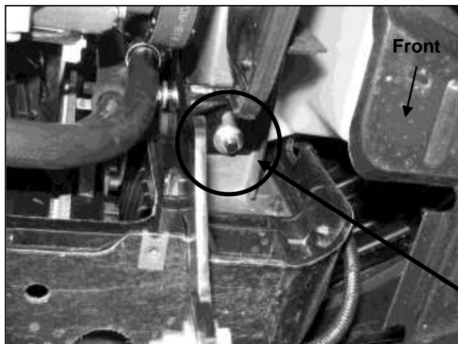
(Fig 7B) Bottom of passenger Frame Bracket attached to Large Bolt Plate pictured from below
