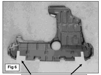
Cut out the sections illustrated to clear the Mounting Brackets (Pictured for example only, actual area to cut may be different)
