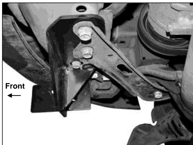
(Fig 3) Passenger/right Mounting Bracket installed
