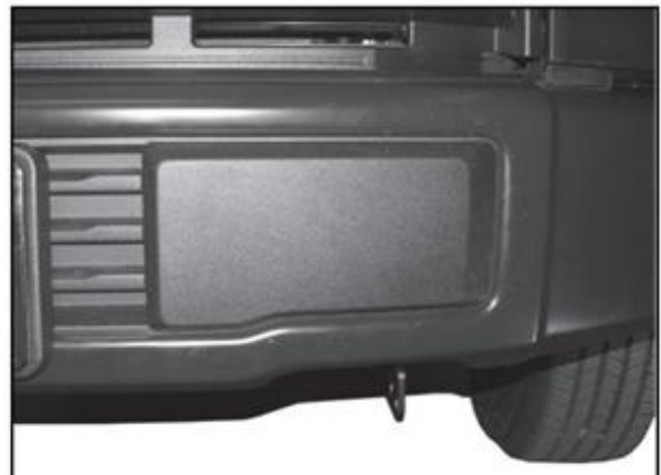
(Fig 5) Remove bumper pads to access splash guard hardware if necessary. 2015 F150 pictured.
