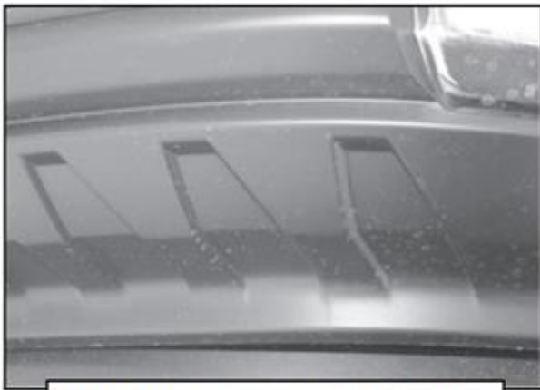
(Fig 4) Temporarily remove the splash guard as required to gain access to the front of the frame channel.
