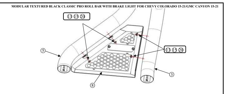
**Step 4:** After the preceding components are preinstalled, connect the side tube and middle tube with standard part 2 .(To adjust tubes to appropriate position, lock tighten all accessories except standard part 2) PS: These adjustable holes can control the width of roll bar.
