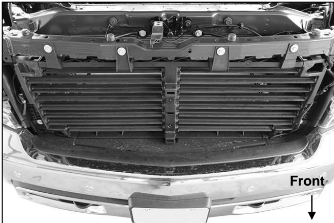
(Fig 12) Remove screws attaching grille and carefully pull grille straight out to remove grille
