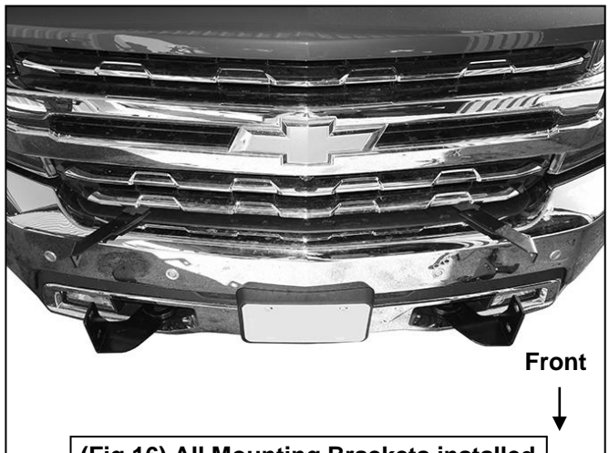
(Fig 16) All Mounting Brackets installed
