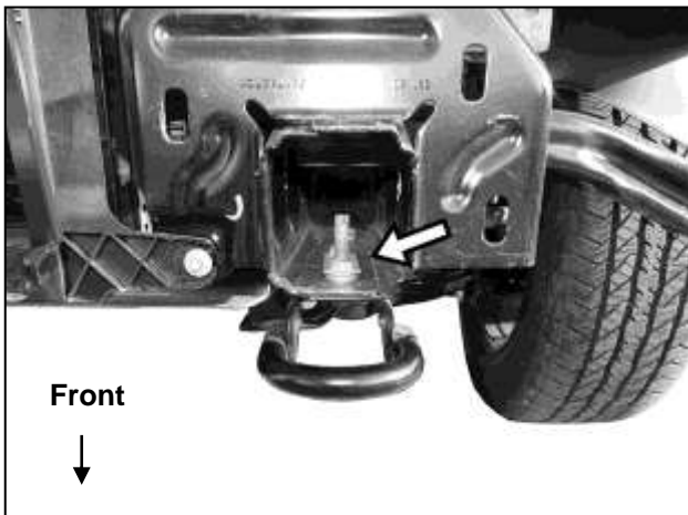
(Fig 8) Temporarily remove tow hooks if equipped
