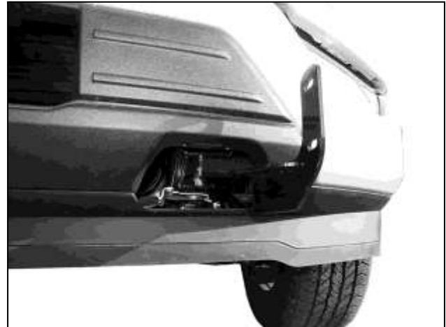
(Fig 12) Driver/left side Mounting Bracket installed without tow hook
