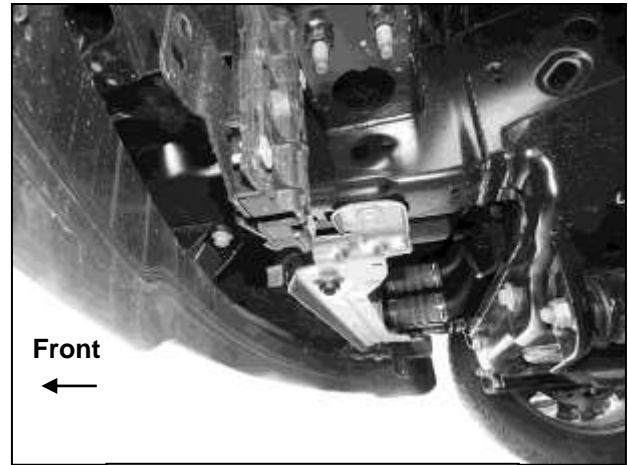
(Fig 2) Active air dam removed
