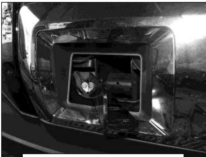
(Fig 4B) Line up holes in Bracket with tow hook mounting holes
