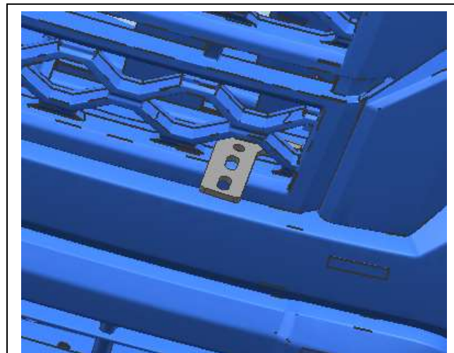
(Fig 4) Attach Driver/Left Inner Support Bracket to vehicle
