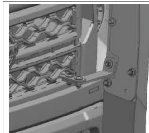
(Fig 7) Attach Driver/Left Outer Support Bracket to Upright
