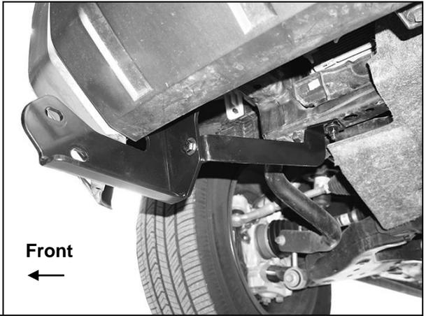
**(Fig 9) Passenger/Right Frame Mounting Bracket and Lower Frame Bracket installed**
