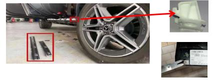
Step 3: Assemble the parts removed from the original car to the new side tread shell as shown in the figure.
