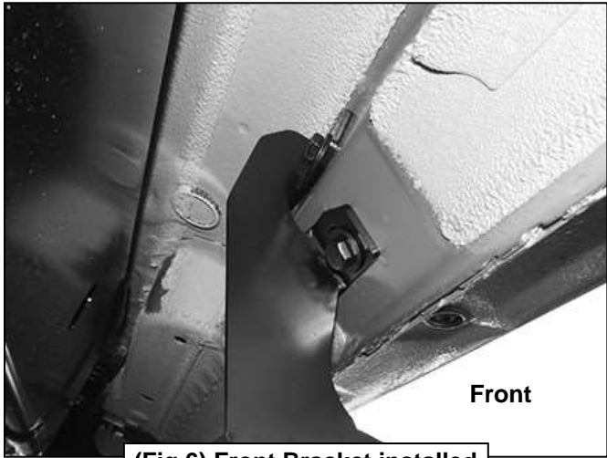
(Fig 6) Front Bracket installed
