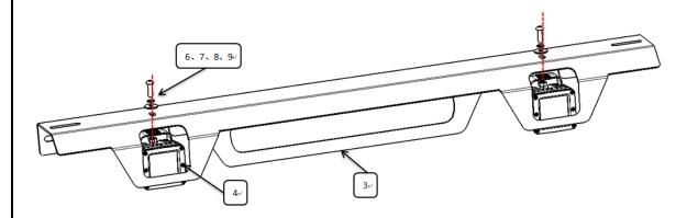
**Step2:** Install (1)(2)(3) and (4) with (6)(7)(8)(9) as below diagram shows.
