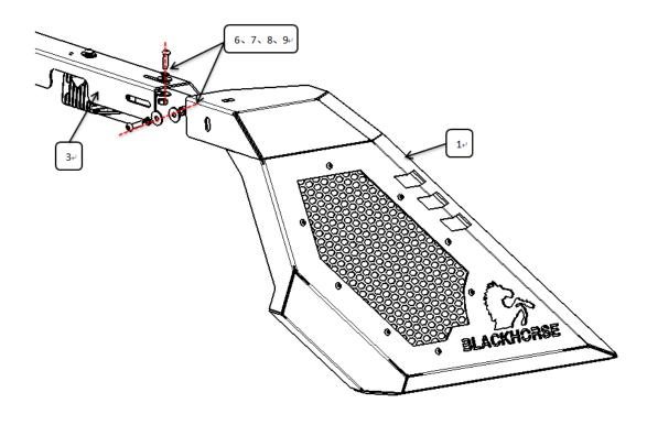
Step 3: Connect brackets and roll bar with standard parts 16 18 19 20 as figure shows.
