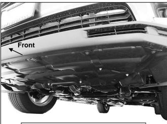
(Fig 1) Remove plastic splash guard
