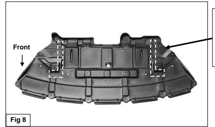
Hold the splash guard up to the bottom of the Brackets. Trace the location of the Brackets onto the inside of the splash guard. Cut (2) openings through splash guard for Mounting Brackets (illustrated for example only. Actual cut out area may differ according to model and year)
