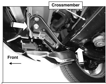
(Fig 2) Passenger side mounting location (arrows)
