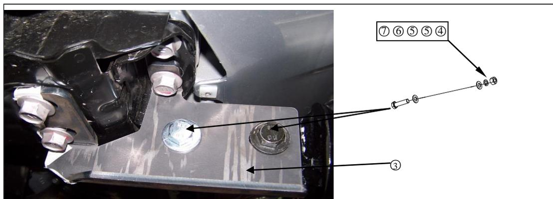
STEP THREE: MAKE SURE BOLTS ARE TIGHTENED AND THE GRILL GUARD IS FIXING STRONG ENOUGH.
