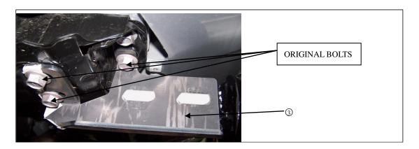
3、INSTALL ① WITH BRACKETS AND TIGHTEN BOLTS. SEE THE PICTURE BELOW.
