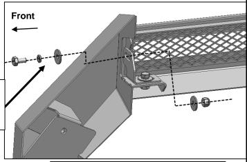
(Fig 6) Driver side light bar Bracket attached to Mesh hardware
