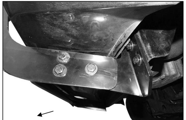
**(Fig 8) Attach Grille Guard to Frame Brackets**
