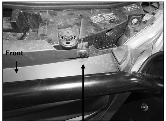
**(Fig 10) Remove factory screw**
