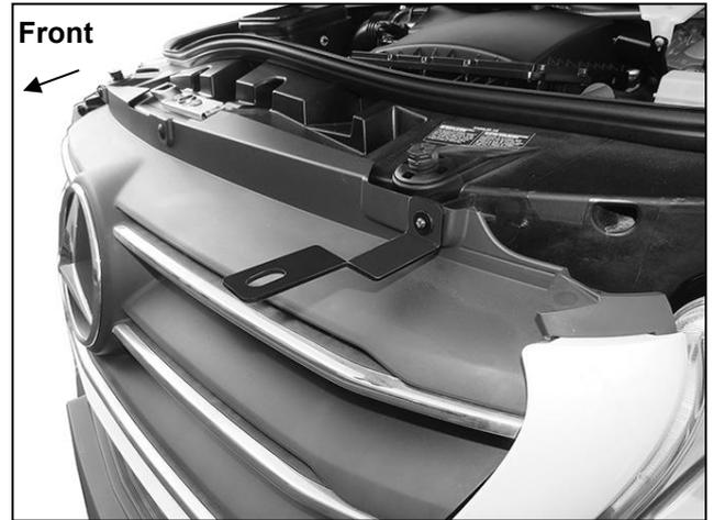
**(Fig 12) Top Bracket installed**
