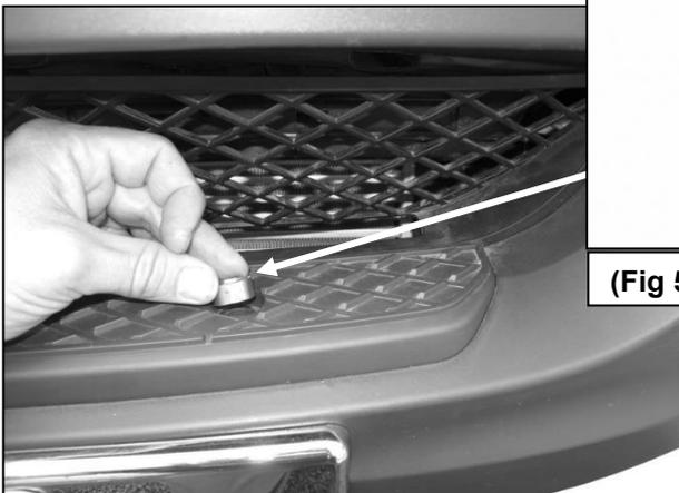
**(Fig 5B) Insert Spacer into recess in bumper**
