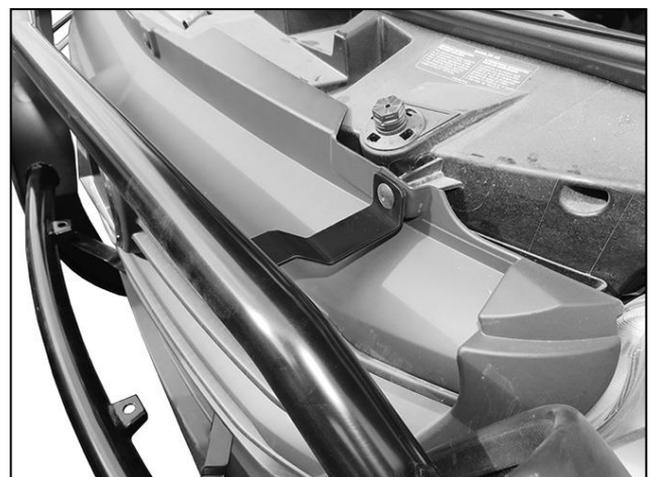
**(Fig 14) Top Bracket installed**
