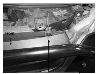
(Fig 10) Remove factory screw
