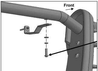
8mm x 25mm Button Head Bolt 8mm Lock Washer 8mm x 16mm Small Flat Washer
