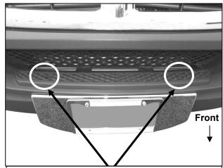
(Fig 4) Remove (2) factory screws (Torx head). NOTE: Remove plastic plugs covering screws if equipped
