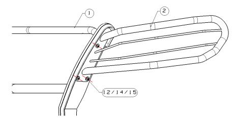
Install Brush Guards and grille guard with standard parts 12 14 15 as below figure shows.
