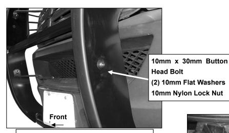
(Fig 9) Attach Center Bracket to upright
