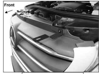
(Fig 12) Top Bracket installed
