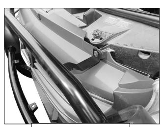
(Fig 14) Top Bracket installed
