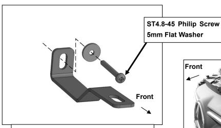
(Fig 11) Attach Top Bracket to top of grille
