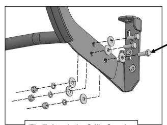
(Fig 7) Attach the Grille Guard to the Driver/Left Mounting Bracket
