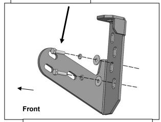
(Fig 2) Attach the Driver/Left Mounting Bracket to the frame
