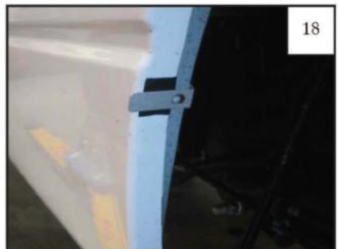
Install a Clip (CL1-0009) over each of the six Tabs (MT1-0014) placed on the sheet metal in Step 17.
