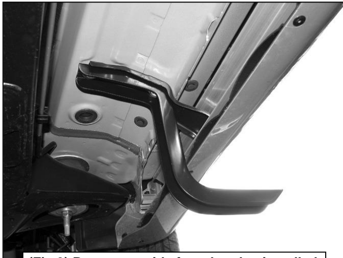
(Fig 3) Passenger side front bracket installed
