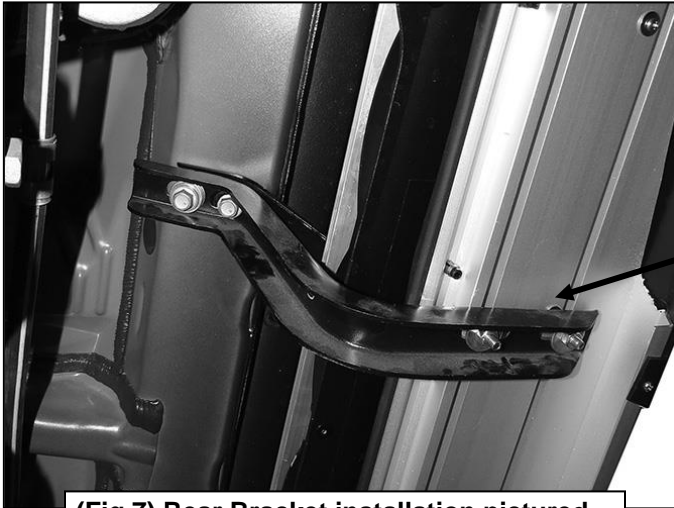
(Fig 7) Rear Bracket installation pictured
