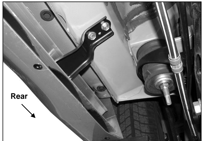
(Fig 4) Passenger side rear bracket location pictured
