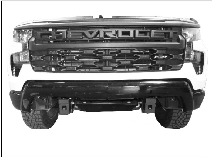
(Fig 22) Reinstall factory grille and upper bumper section to vehicle.
