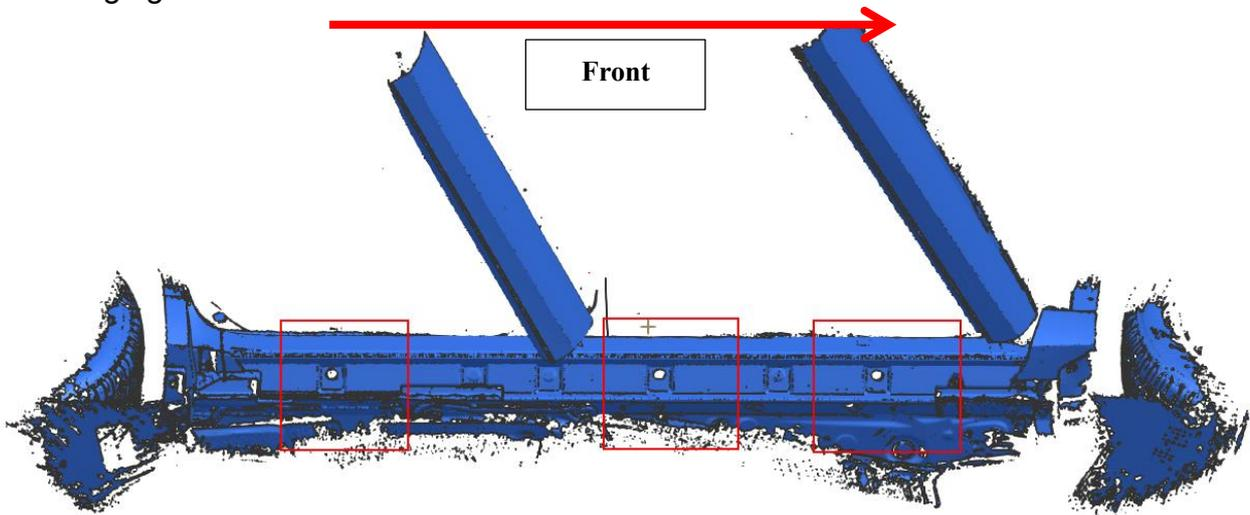
Step 3: Use standard parts to fix the Passenger/Right Front Mounting Bracket to the vehicle body, and the installation method is as follows. The installation method on the left side is consistent.
