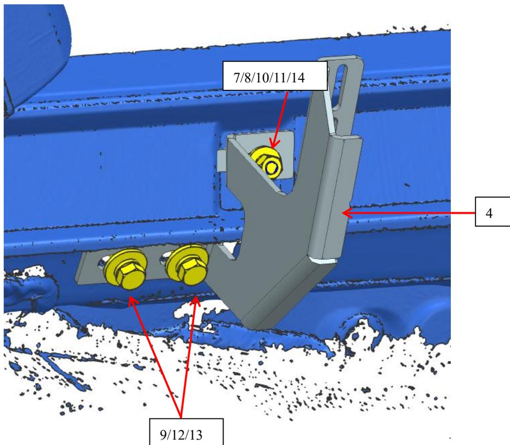
Step5: Use standard parts to fix the Passenger/Right Rear Mounting Bracket to the vehicle body, and the installation method is as follows. The installation method on the left side is consistent.
