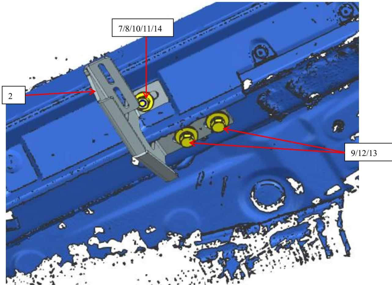
Step 4: Use standard parts to fix the Passenger/Right Center Mounting Bracket to the vehicle body, and the installation method is as follows. The installation method on the left side is consistent.
