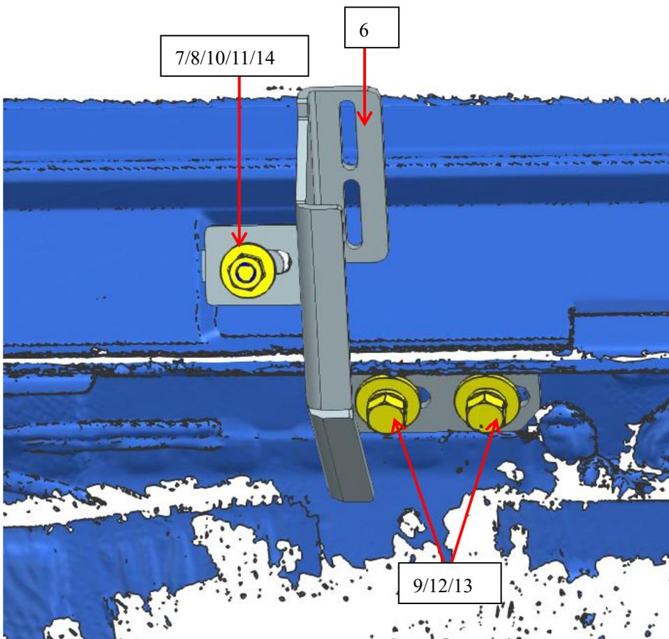
Step6: Place the right running board on the installation surface of the right side of front bracket, center bracket and rear bracket. Adjust the appropriate position, and use the small square head bolts on the running board and corresponding standard parts to lock and install the right running board with the right side brackets. Install the left running board symmetrically.
