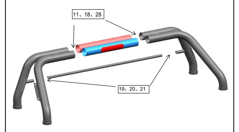
Step 2: Using wrench 15, install 1/2 main pipes and connecting plate 5 together with parts 9/ 10/11/13 as shown.
