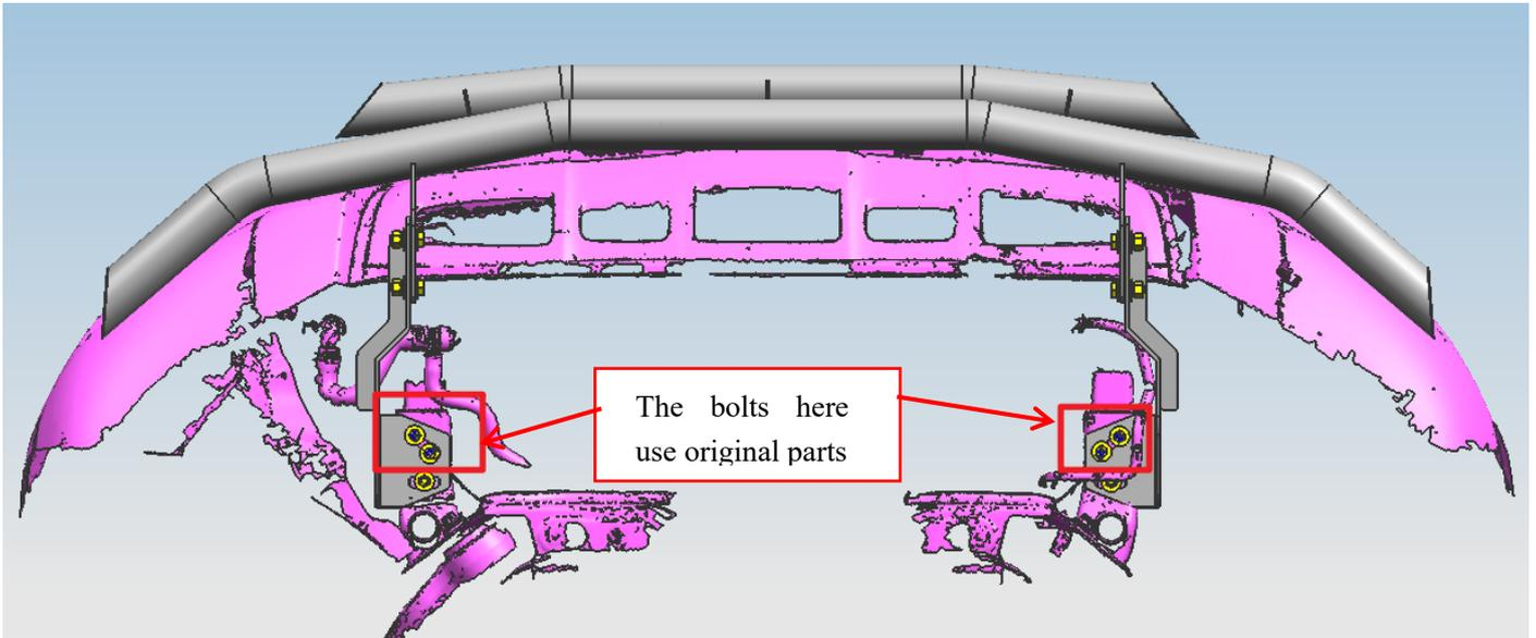
Step 3: Install the bull bar on the brackets and then adjust them to the proper positions.
