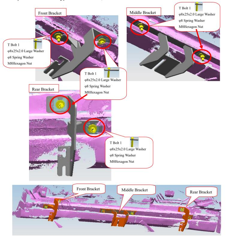
Step 3: Install the running boards on the brackets and then adjust them to the proper positions.
