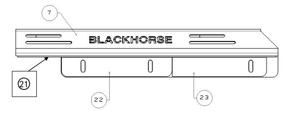
**Step3:** Connect the roll bar with mounting base by ha standard parts 9001/23
