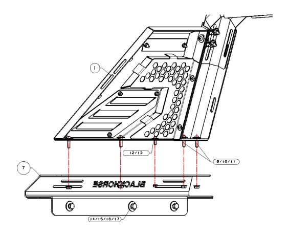
**Step 4**: Install roll bar on truck rail by hard standard parts 4 15 16 17
