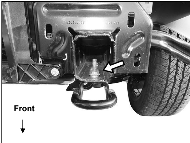
(Fig 8) Temporarily remove tow hooks if equipped
