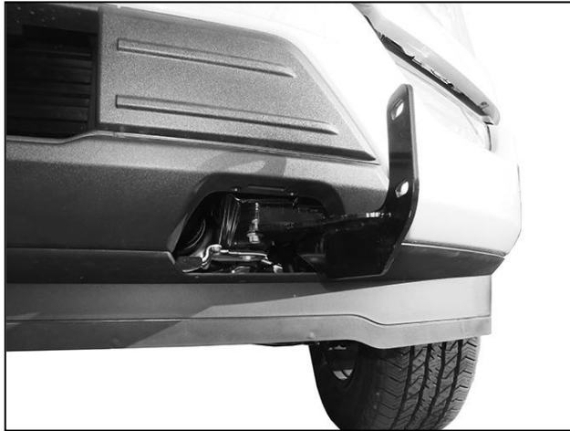
(Fig 13) Driver/left side Mounting Bracket installed without tow hook
