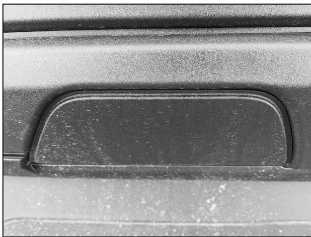
(Fig 10) On models without tow hooks, release clips and remove plastic covers
