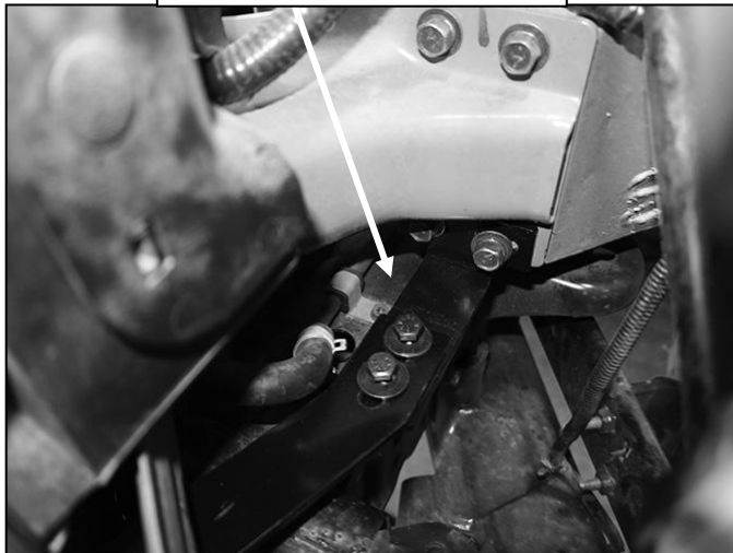
(Fig 11) Slide Top Support Bracket through bumper, (see Fig 12). Attach Bracket to top of Mounting Bracket
