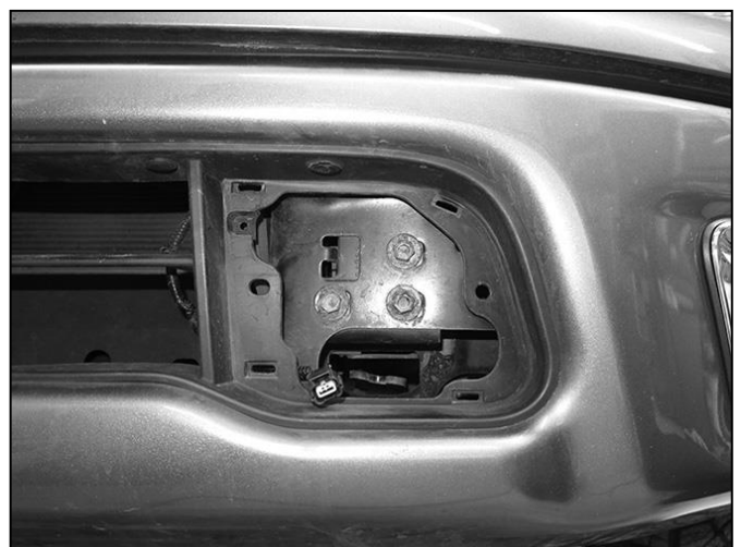
(Fig 2) Remove plastic panel. Models with parking sensors, unplug harness
