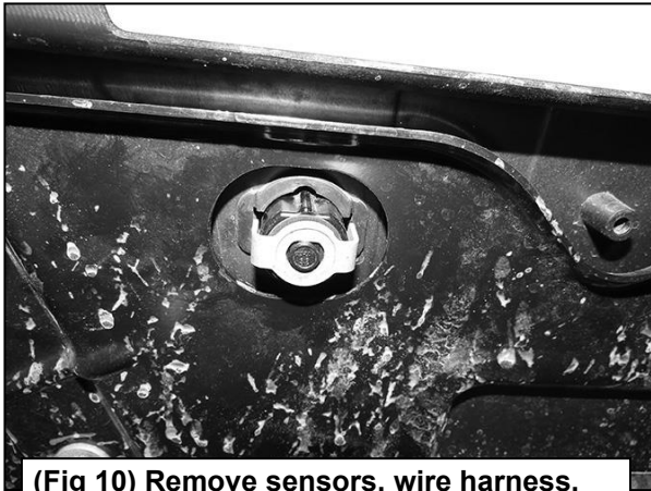
(Fig 10) Remove sensors, wire harness, license plate lights, trailer plug and spare tire access lock (pictured) if equipped
