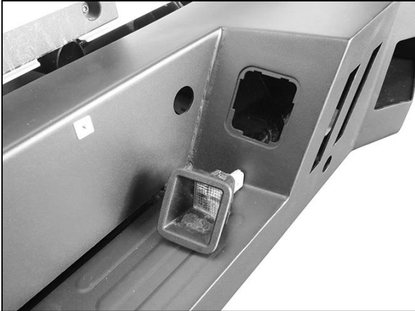
(Fig 15) Push license plate lights into openings and plug into bumper wiring harness
