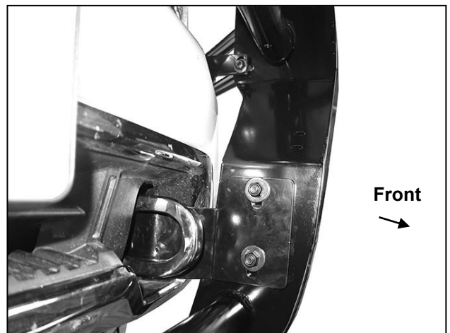
(Fig 18) Grille Guard installed (driver/left side pictured)
