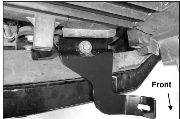
(Fig 7b) 2024-on: Reuse bumper bracket bolt to attach Driver/left Top Bracket to top of frame
