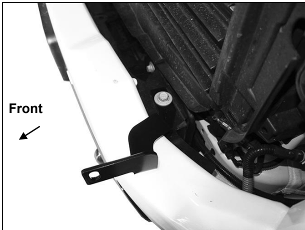
(Fig 7a) Reuse bumper bracket bolt to attach driver/left Top Bracket to top of frame
