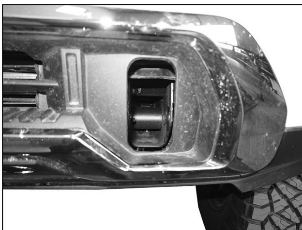
(Fig 10) Reinsert tow hook. Insert driver/left outer Frame Bracket through opening and along outside of frame
