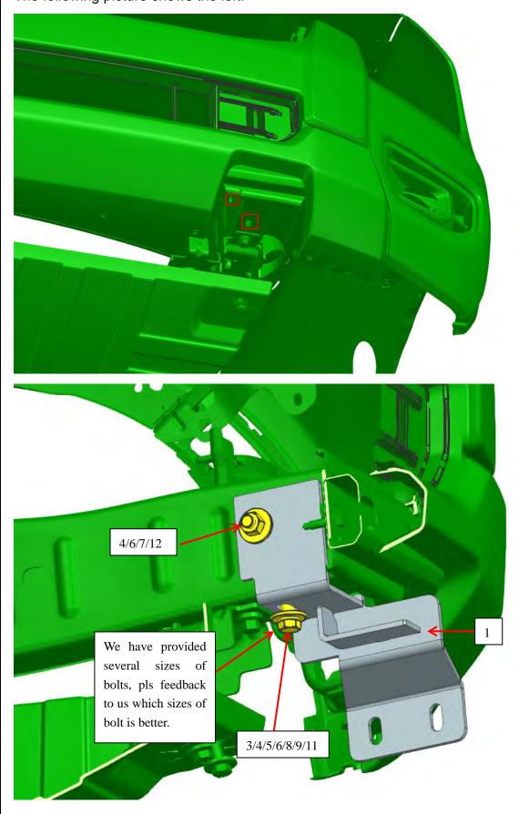
Step 3: Install and fix the grille guard and brackets using standard parts, as shown in the following figure:
