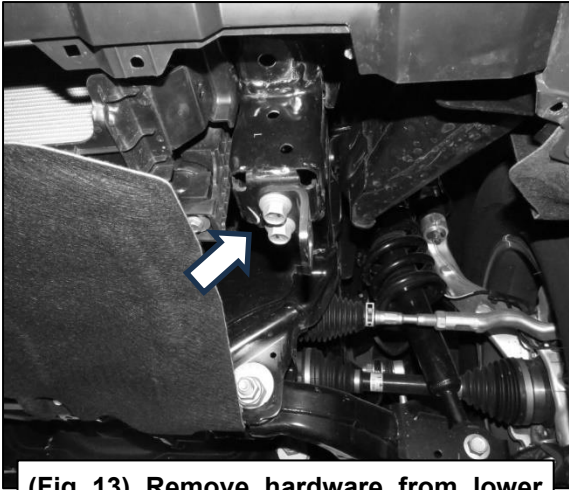
(Fig 13) Remove hardware from lower Frame Mounting Bracket mounting point
