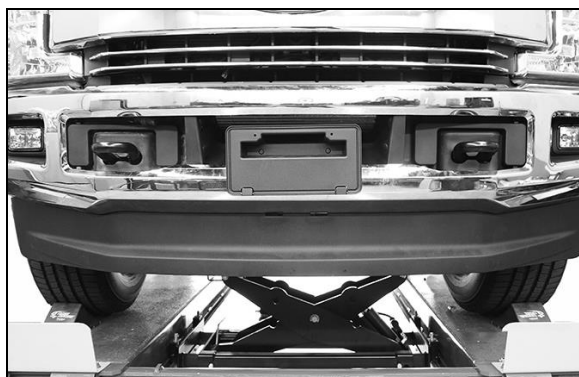
(Fig 5) Remove plastic air dam from bottom of bumper.
