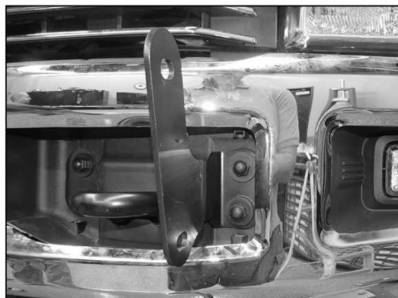
(Fig 4) Reuse factory bumper bolts to attach driver/left Upper Bracket to bumper
