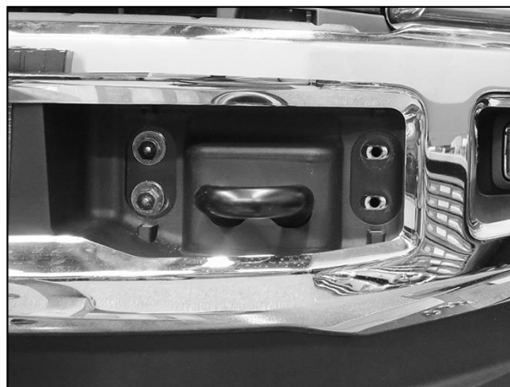
(Fig 2) Remove outer bumper bolts only
