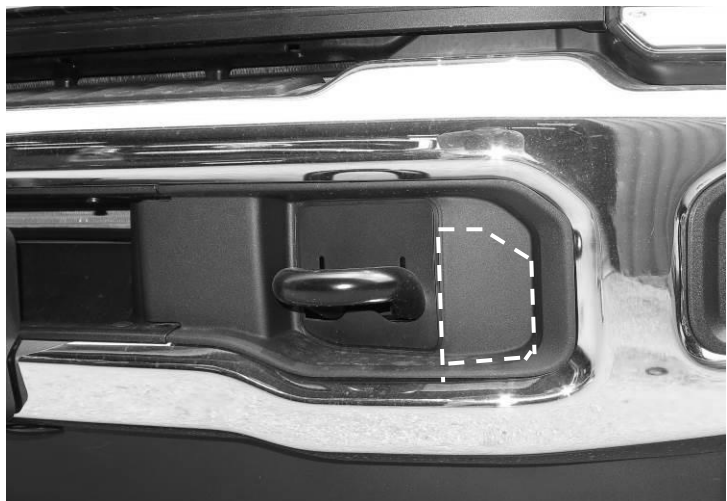
(Fig 1) Remove cover over bumper bolts.
