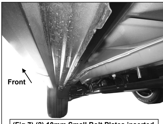
(Fig 7) (2) 10mm Small Bolt Plates inserted into the center mounting location
