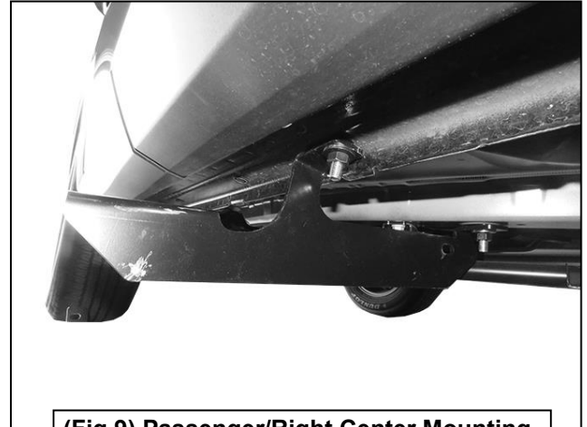
(Fig 9) Passenger/Right Center Mounting Bracket attached to the (2) Bolt Plates
