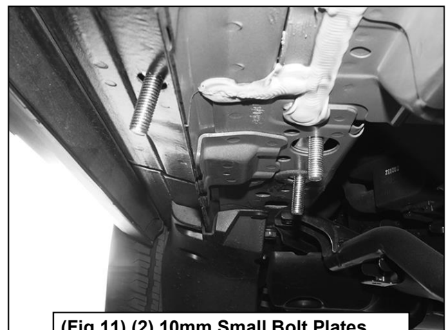
(Fig 11) (2) 10mm Small Bolt Plates and (1) 10mm Large Bolt Plate inserted into the rear mounting
