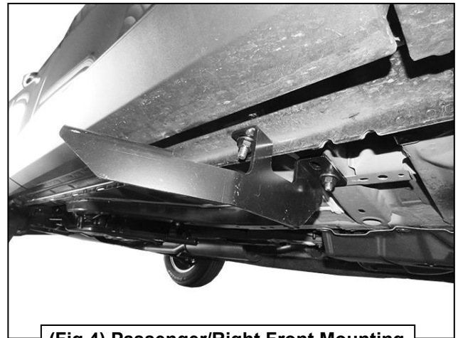
(Fig 4) Passenger/Right Front Mounting Bracket attached to the (2) Bolt Plates
