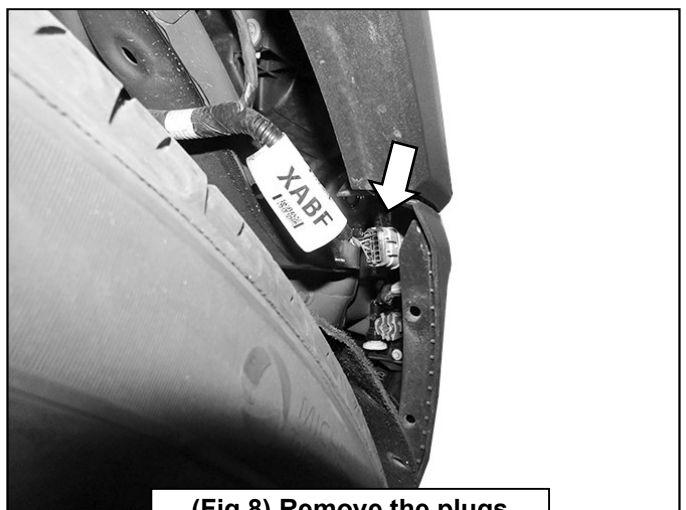
(Fig 8) Remove the plugs inside the fenders
