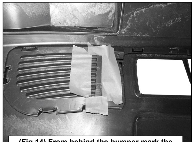
(Fig 14) From behind the bumper mark the indicated area with tape and with a hacksaw or sharp knife, make small cuts
