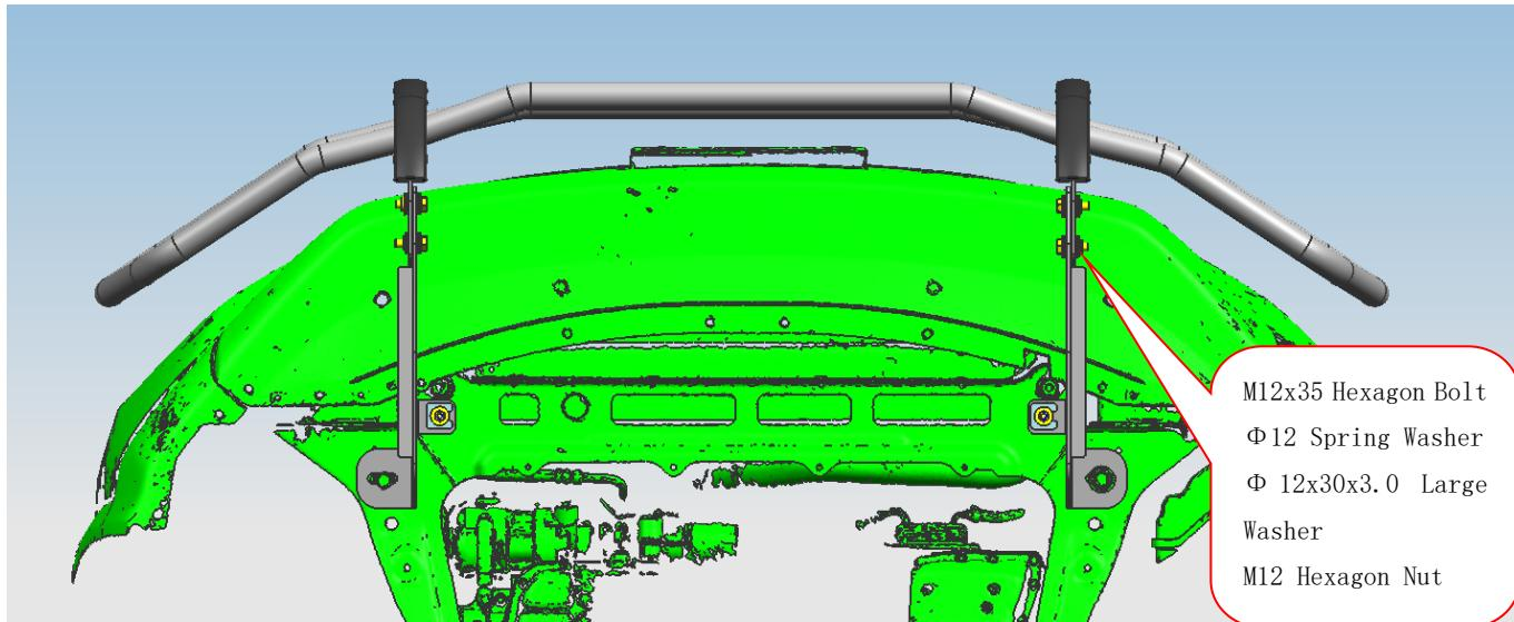
Step 4: Check if all hard ware are installed and then fasten all to complete the installation.
