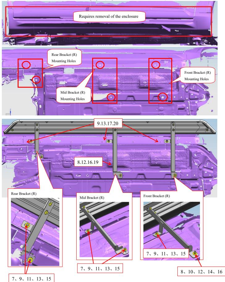
Step 3: Install the pedal on the bracket and adjust the installation position of the bracket according to the position of the pedal.
