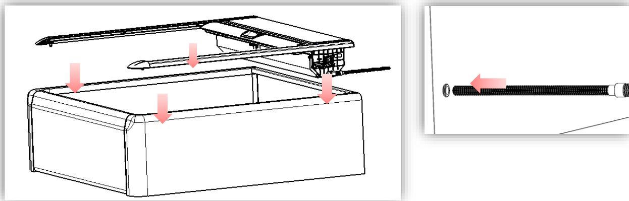
7. Put the rubber foam ② on the tailgate, as the photo shows above. Close the roller lid and pull it backwards until it touch the rubber foam.
