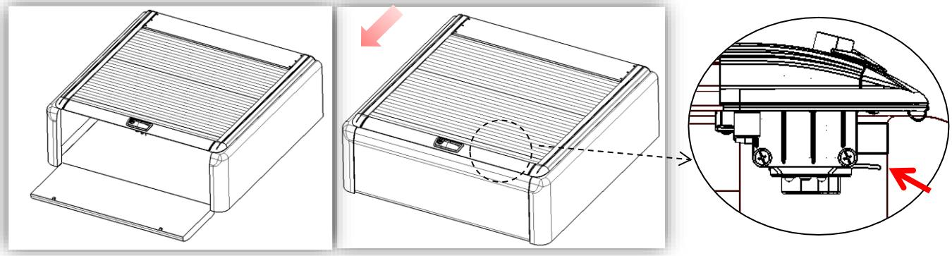
8. Open the roller lid and put the ⑩ standard bar to adjust the width between two side rails. Distance between the side rails should be same from front to rear part.
