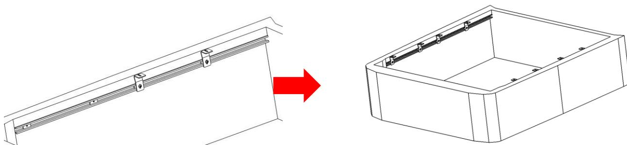
11. Install the drain-tube ⑥ at the rear part of the side rail. (Both sides should be same)
