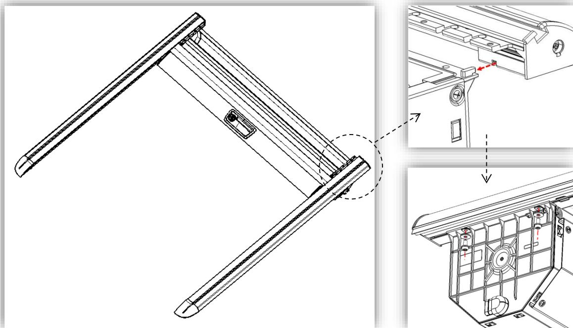
3. Install the drain-pipe (7), assembly way is same on both sides.
