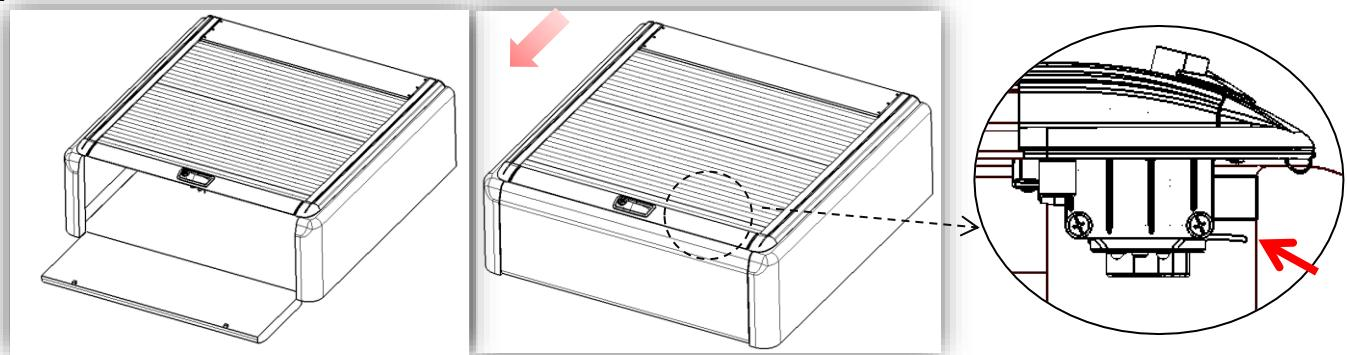
8. Open the roller lid and put the ⑩ standard bar to adjust the width between two side rails. Distance between the side rails should be same from front to rear part.
