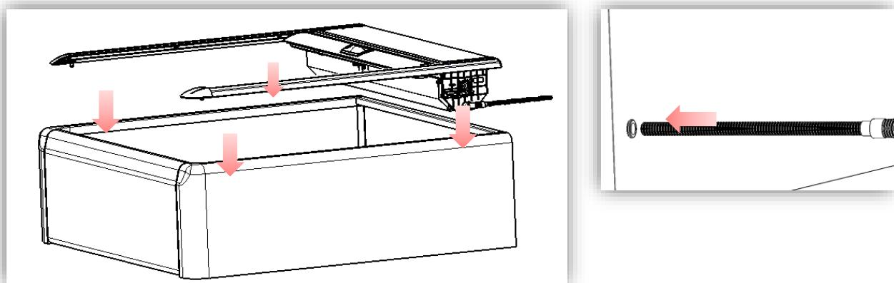
7. Put the rubber foam ⑨ on the tailgate, as the photo shows above. Close the roller lid and pull it backwards until it touch the rubber foam.
