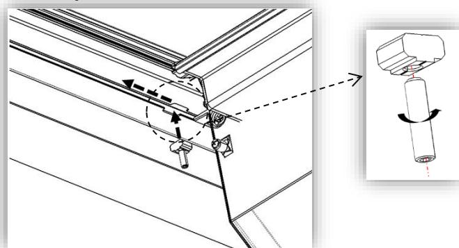
10. Install the ⑫ clamps and put it to appropriate position, fasten it with ⑪ M6 bolt combo.
