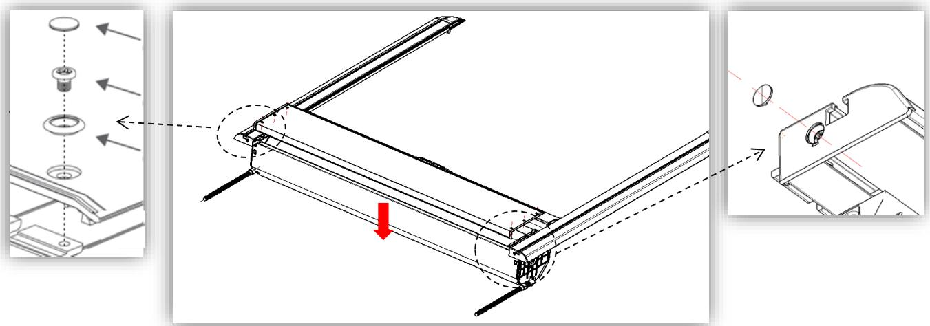
5. Find the two holes on the front of the truck bed, and then install the grommet ⑦ on it. Both sides should be same. Install the bulkhead seal ⑧ and trim it at the corner part to match the side rails.
