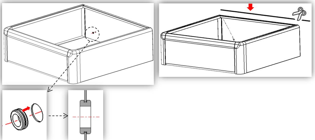
6. Put the roller shutter on truck bed, thread the front drain-tube to the truck bed.
