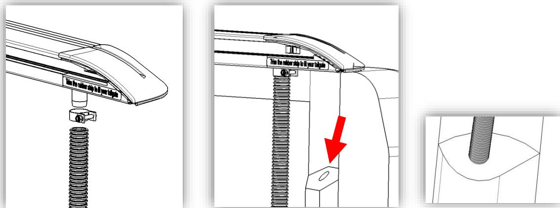
**12. Install the ⑨ end cap on tailgate; fix them with the self-tapping screws. (as the picture shows below).**
