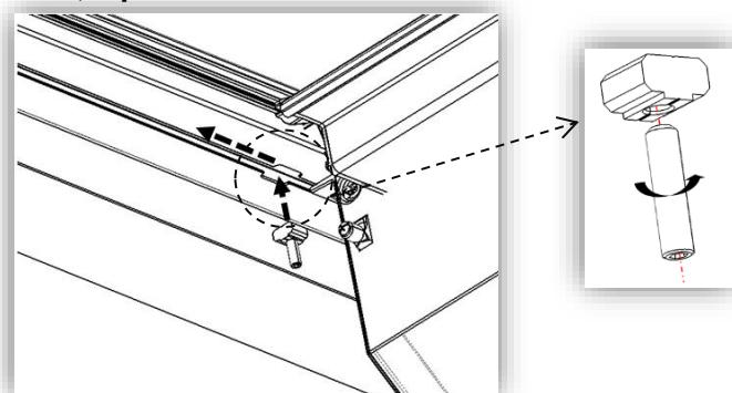
10. Install the ③ clamps and put it to appropriate position, fasten it with ① M6 bolt combo.
