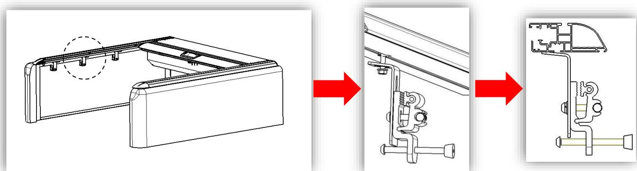
**11. Install the drain-tube ⑥ at the rear part of the side rail. (Both sides should be same)**
