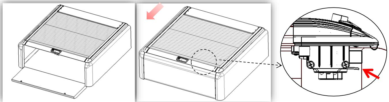
8. Open the roller lid and put the ⑥ standard bar to adjust the width between two side rails. Distance between the side rails should be same from front to rear part.
