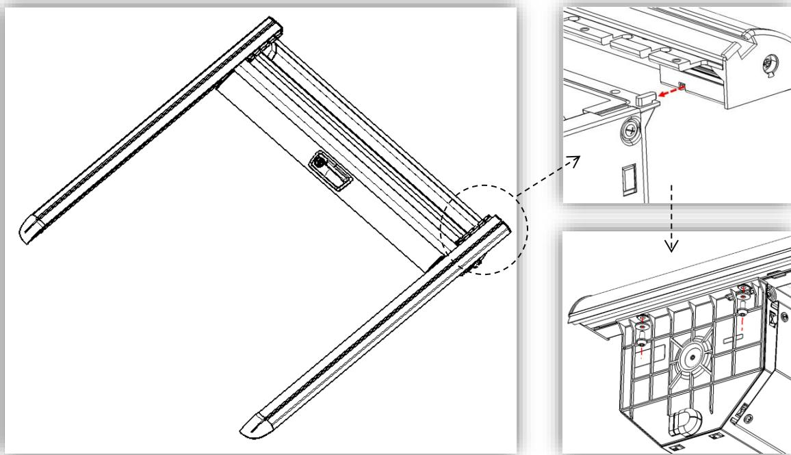
3. Install the drain-pipe **⑦**, assembly way is same on both sides.
