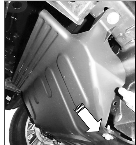
(Fig 2) Remove factory bolts attaching bottom of splash guard (arrow). Upper cover pictured
