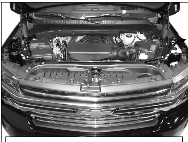
(4-1) Remove plastic cover from top of grille
