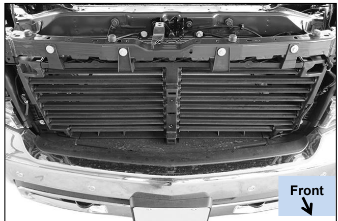
(4-2) Remove screws attaching grille and carefully pull grille straight out to remove grille
