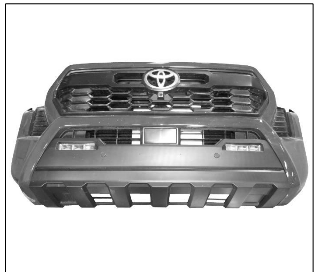
(Fig 6) Pull Bumper from sides and forward to detach from vehicle
