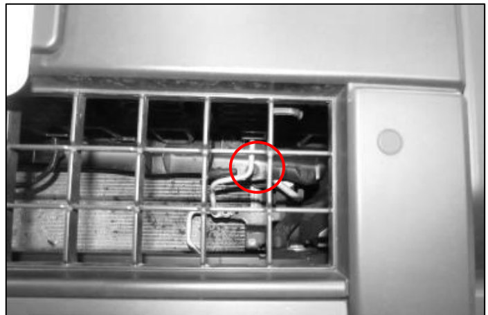
(Fig 9) Locate the Driver/Left Support Bracket mount point circled and remove the bolt.
