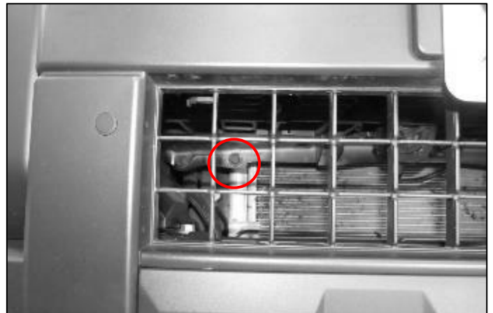
(Fig 7) Using a ratchet extension, remove the bolt from the Passenger/Right Support Bracket mount point and set it aside. In the case of dropping the bolt into the front fascia, it is recommended that you have a magnet to retrieve the bolt.
