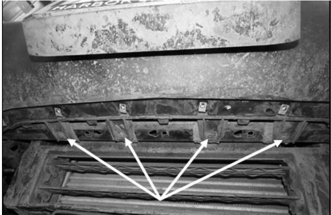
(Fig 6) Remove the 4 torx bolts at the bottom of the bumper
