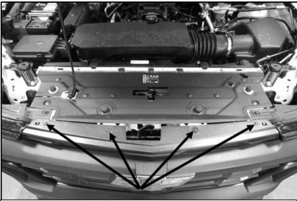
(Fig 5) Remove the 4 torx bolts at the top of the grille underneath the hood
