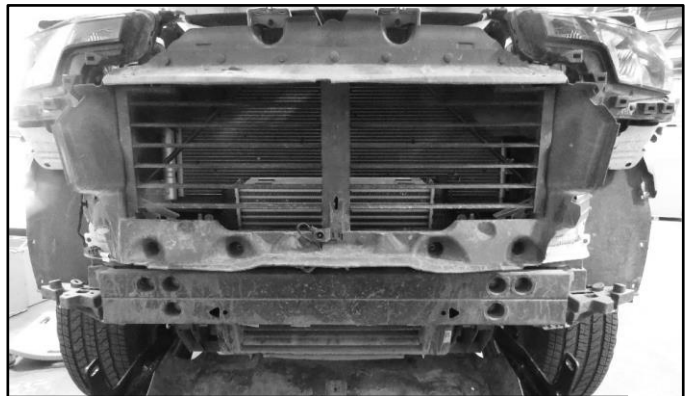
(Fig 8) Remainder of the fascia removed
