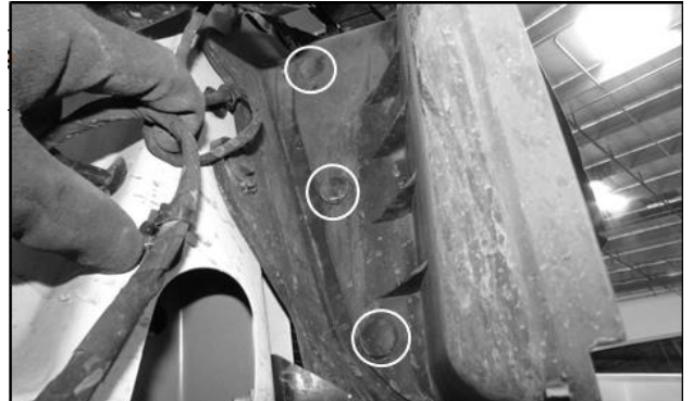
(Fig 10) Remove the clips on the sides of the shroud
